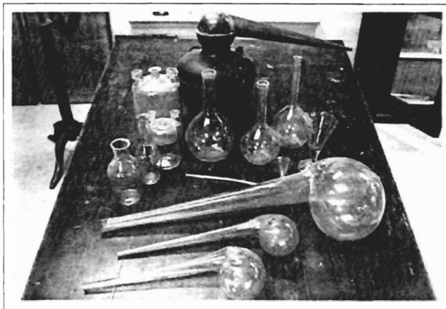
A selection of the chemical apparatus, including Woulfe bottles, gas-generating bottles, flasks, retorts and a precipitation glass
