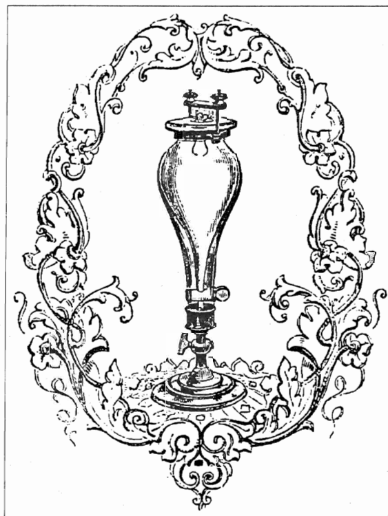
Logo of the Cavendish Society: Henry Cavendish's glass eudiometer for sparking gas mixtures
