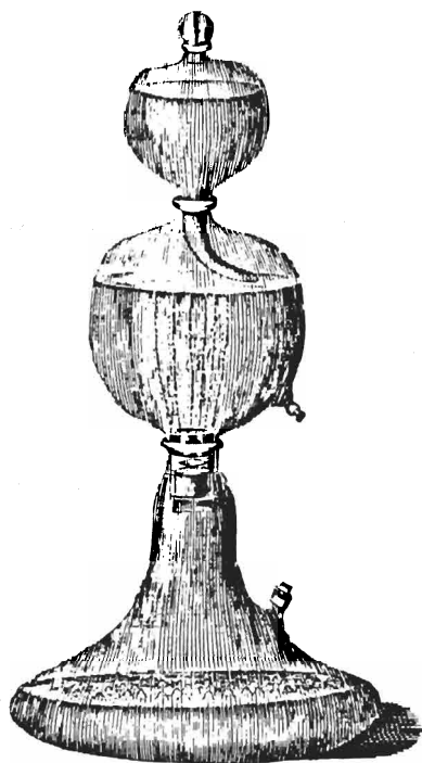
A Nooth apparatus used by Mrs Fulhame in her experiments. Originally made to carbonate water, gases chemically generated in the lower chamber are bubbled through the liquid in the upper chamber, where they can react with the liquid or with various solutes.
