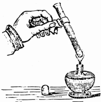
A paper twist test tube clamp, circa 1850 (1)
