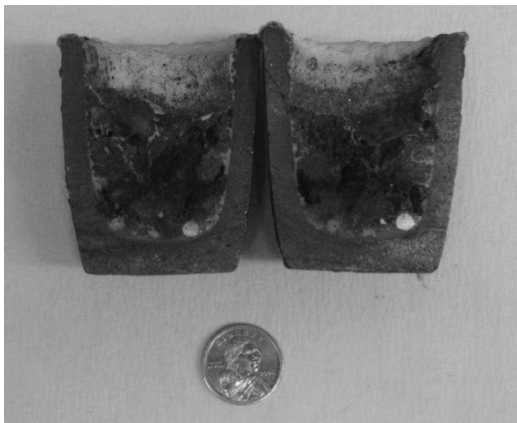
Figure 1. A graphite crucible cut in half following a modern demonstration run on the small scale. Halves of shiny aluminum globules are in the bottom of the crucible.
