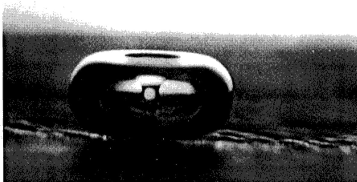
Fig. 3. Liquid jet produced during collapse of a cavitation bubble near a solid surface. The width of the bubble is about 1 mm. Reproduced with permission (8).
