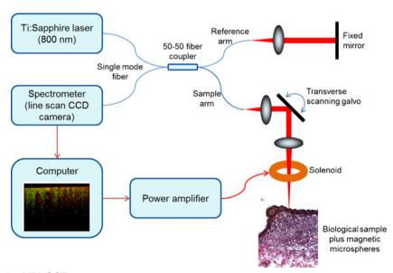
Fig. 3. Schematic of the MM-OCT system.
