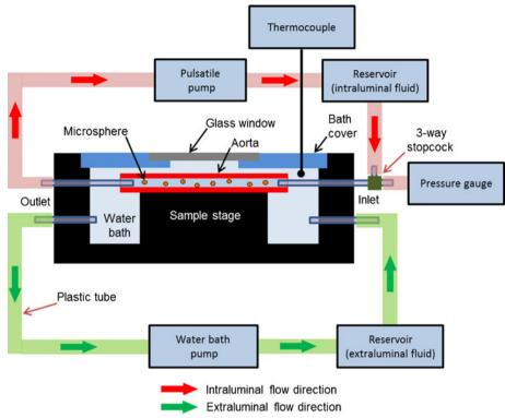
Fig. 2. Schematic of a custom-built flow chamber used for perfusing *ex vivo* aorta segments. The flow chamber consisted of a Plexiglas water bath container for extraluminal fluid (PBS). Each aorta segment was mounted between the plastic inlet and outlet tubes inside the chamber, whereas a pulsatile high-pressure blood pump was designed to replicate the *in vivo* conditions in a rabbit.
