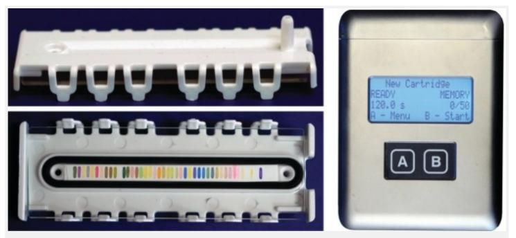
This optoelectronic "nose" (side and front views, left) and handheld reader-analyzer (right) detects TATP and many other compounds on the basis of the response of an array of colorimetric sensors embedded in a disposable cartridge.
