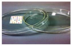
A colorimetric sensor array is placed in an Petri dish for culturing bacteria and scanned with an ordinary flatbed photo scanner kept inside a lab incubator. The dots change color as they react with gases the bacteria produce. Photo by K. S. Suslick
