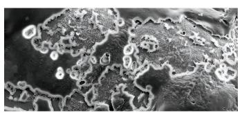
PTFE coatiing on an NaCl crystal degraded by ultrasonic heating
