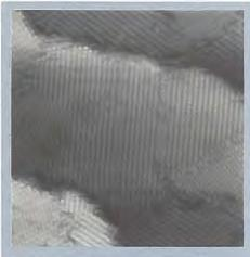
Figure 1. Complex patterns are observed that reflect an interplay between the metal lattice structure, the structure of the silicotungstate anion, and the resultent edlayer structure.
