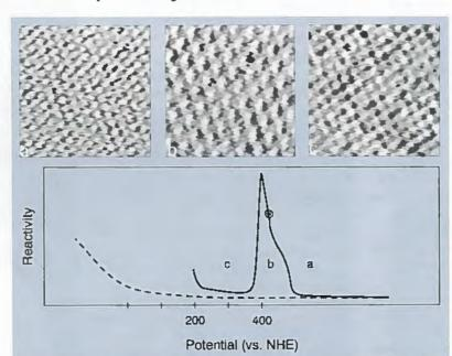
Figure 2a: AFM images (5 x 5 nm) of Bi upd on Au(111) in 0.1 M HClO4. a) Au(111) surface found positive of Bi upd peaks, b) (2 x 2)-Bi adlattice found at +200 mV of bulk deposition. Atom-atom distance is 0.57  $\pm$  0.02 nm. c) Uniaxially commensurate rectangular Bi adlattice found at 100 mV. Atom-atom distance is 0.34  $\pm$  0.02 nm. 2b: Reactivity plot of deposition stages.
