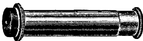
A pocket spectroscope. Circa 1925.
